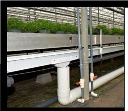
Closed systems may include technologies like these flood benches and troughs, which collect nutrient feed water for reuse.
